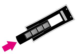
6 Place the XPA light source into the positioning plate with negatives facing down and the HP logo facing you.
